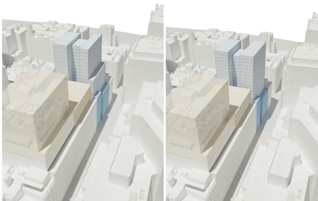
Figures 25 and 26 – aerial view from north showing 8m tower setback above Red Cross House addition (left) and proposed 4m tower setback (right)
